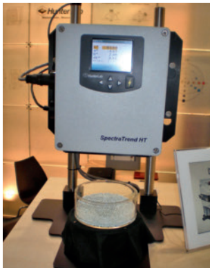
Fig. 7. Hunterlab SpectraTrend for use with plastic pellets (photo: Schröder)
