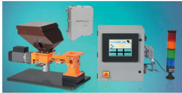
Fig. 6. Online color monitoring and control system (photo: X-rite Inc.)
