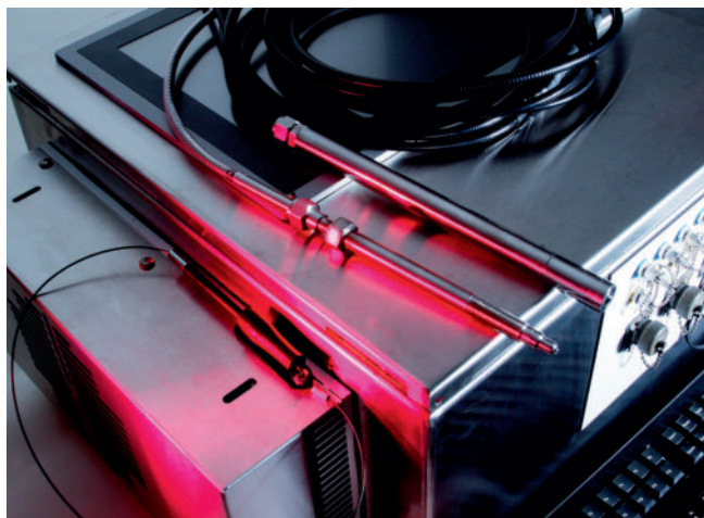
Fig. 5. RPMP measuring probe for installation in an extruder (photo: ColVisTec, Berlin)
